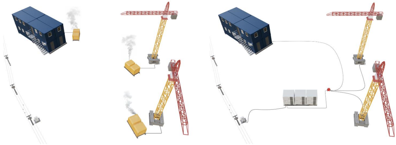
Figure 1: Construction site powered by diesel generators (left); construction site powered by a Voltpack Mobile (right)
